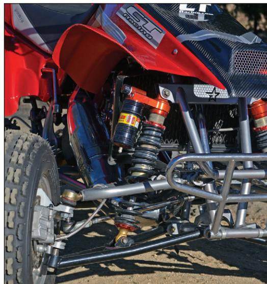
*The stock suspension on the Honda 250R was better than the competition, but by 1990, the top racers were all using aftermarket equipment to get an advantage. The JB Racing/Elka combo installed on this project is still better than some stock front ends found today.*
