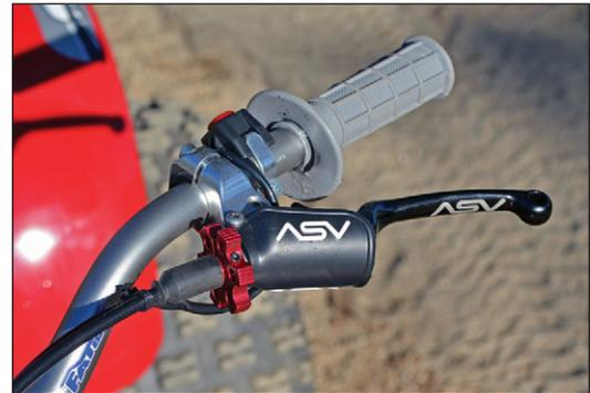
**On the new Rental handlebars we installed a Motion Pro twist throttle and a pair of Pro-series F3 folding levers from ASV Inventions.**
