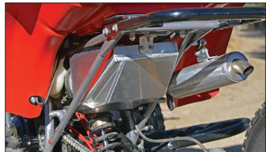
**For this project we replaced an old stock plastic airbox with a clean aluminum unit from CM Performance. Inside a Twin Air foam filter replaced an older single-layer foam unit.**
