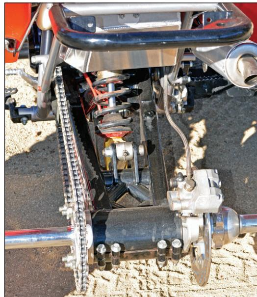
*Back in the day the trick was to get the suspension to work well enough to soften the ride and not destroy the frame and swingarm. Arens and JB Racing came up with super-strong components that could hold up to any abuse.*
