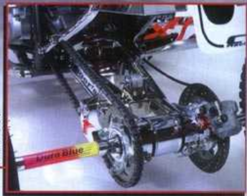
A +1.5" Laeger swingarm and Durablu +4" axle give the 400 a race ready stance.
