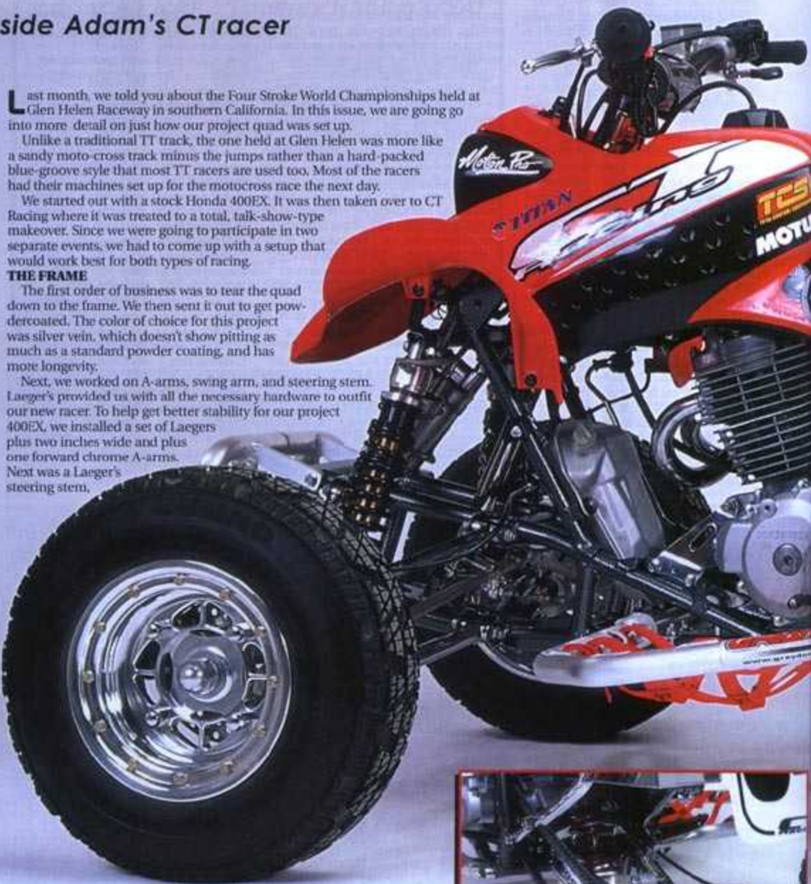
A +1.5" Laeger swingarm and Durablu +4" axle give the 400 a race ready stance.
