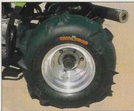
The Kenda Sand Gecko paddle tires are mounted on lightweight aluminum Douglas wheels. The combination is four inches wider than stock.
