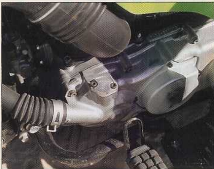
CT Racing's Complete Power Package is awesome, but you do lose the oil injector. Premixed race gas is required.
