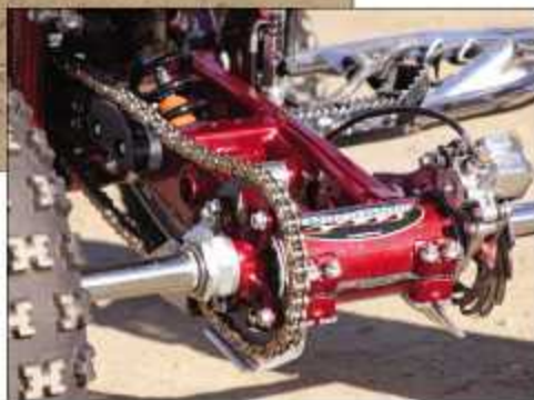
The stock swingarm was used in conjunction with the Race Tech shock. It handled whoops and jumps with aplomb.
