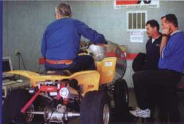
A couple of interested spectators look on as Dennis Mahan puts our pipe contestants through several runs on the K&N dyno.
