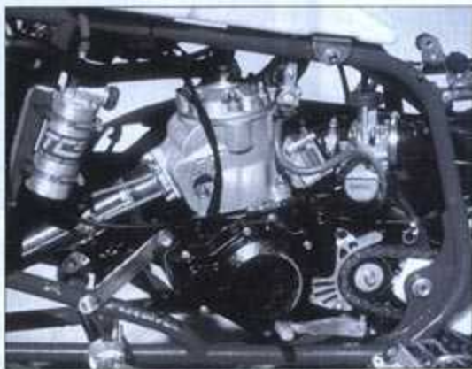
Both engines are big-bores, consisting of 350cc of raw two-stroke power. They also feature Pro-X Interchangeable Domes and a 38mm PWK Air Striker carburetor.
