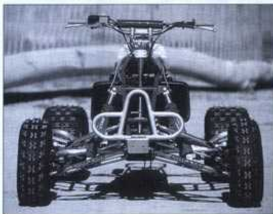
Racing quads are all about function. Weight is saved on these aftermarket frames by eliminating unneeded tabs and mounts.
