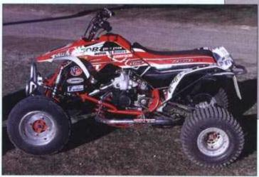
The black round thing you see sticking out of the front of the top of the cylinder is the diaphram cover for the RAVE valve. CT Racing machines the cylinder (with no welding) to accept the RAVE valve. It is the same system used in Bombardier's See-Doo watercraft and Ski-Doo snowmobiles.
