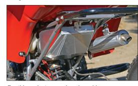
For this project we replaced an old stock plastic airbox with a clean aluminum unit from CM Performance. Inside a Twin Air foam filter replaced an older single-layer foam unit.
