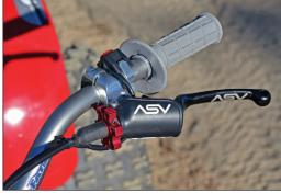
On the new Renthal handlebars we installed a Motion Pro twist throttle and a pair of Pro-series F3 folding levers from ASV Inventions.
