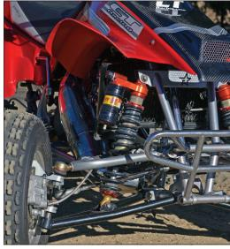
The stock suspension on the Honda 250R was better than the competition, but by 1990, the top racers were all using aftermarket equipment to get an advantage. The JB Racing/Elka combo installed on this project is still better than some stock front ends found today.
