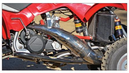
No electric starter here or dead-battery fears. A solid kick will get this machine up and running easily with significant weight savings.
