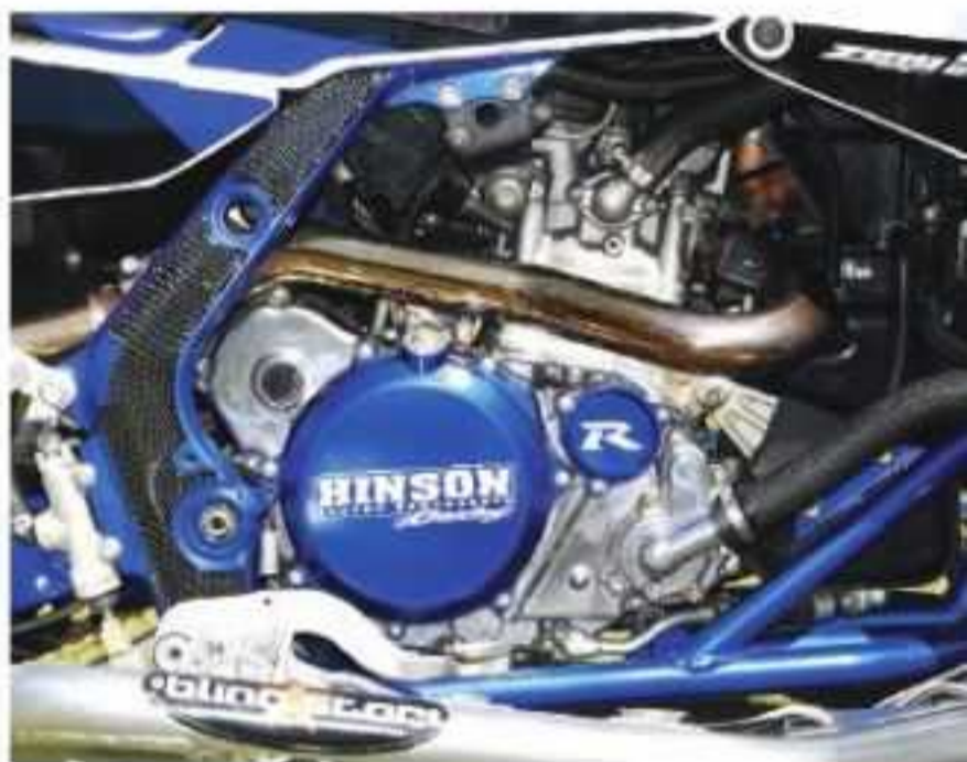
The JE Pistons 13.5:1 piston requires race gas and boosts power with the degreed Web cams and Dynatek Power Commander. All the extra braking power is reduced to manageable by the Hinson slipper clutch.
