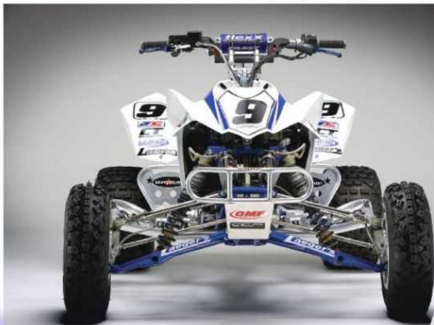
Laeger Pro Trax front A-arms eliminates ball joints for more and smoother travel, and the Elka 3 steering damper cuts out after 20 degrees of turn angle, so you don't fight the damper when cranked sideways in turns.
